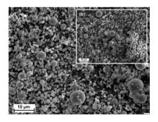
Fig. 7. SEM images of the pigments obtained by adsorption of C.I. Basic Blue 9 in concentration of 3000 mg/dm<sup>3</sup> on (a) unmodified and (b) modified TiO<sub>2</sub>–SiO<sub>2</sub> support
