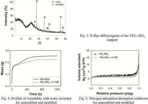
(3 wt./wt. of U-15D) TiO<sub>2</sub>-SiO<sub>2</sub> composite
