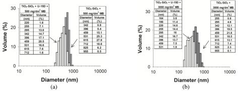
Fig. 6. Comparison of the particle size distributions according to volume contributions evaluated for the pigments obtained by adsorption of C.I. Basic Blue 9 in concentration (a) 500 mg/dm<sup>3</sup> and (b) 3000 mg/dm<sup>3</sup> on unmodified and functionalized TiO<sub>2</sub>–SiO<sub>2</sub> support
